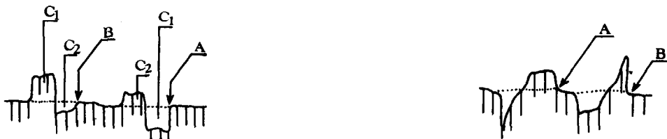
Fig. 2. Example of ghost zones. Columns: Separon Six CN. Eluent: THF-water (80:20, v/v). Elution rate: 0.3 ml/min. Pressure: 6 MPa. Sensitivity of detector: 16 \times . Counts: 15 drops of effluent, i.e. , about 0.4 ml. A, Recycling valve R switched from position b to a. B, valve R switched from position a to b; C 1 , zone from column C 1 ; C 2 , zone from column C 2 .
